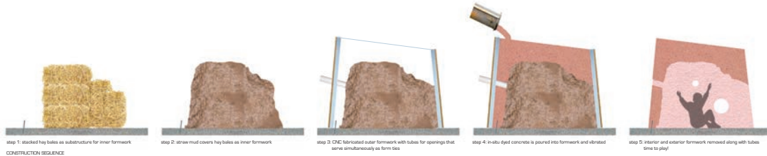
step 1: stacked hay bales as substructure for inner formwork
